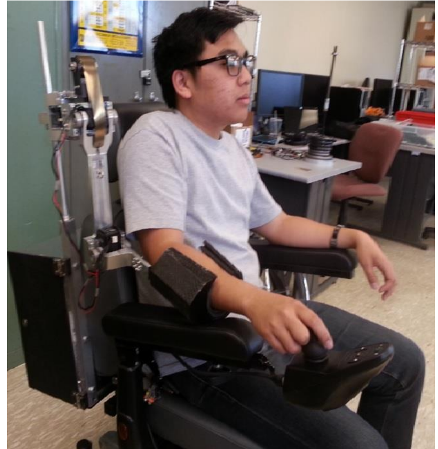
Robotic arm attached to wheelchair with user.
